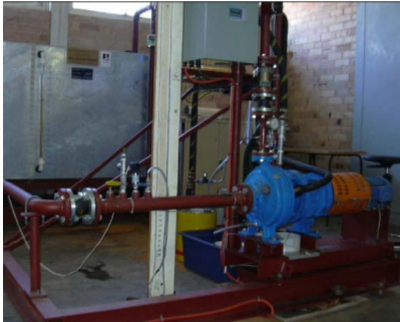
**Figure 4:** Thermo fluid pump rig
