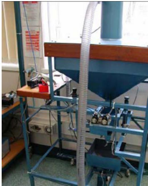
**Figure 3:** Sand-weighing machine (e-Laboratory Hardware).
